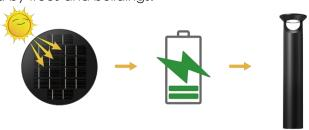
It is available with automatic activation (PWM controller) to save energy and last longer. The operating hours can be divided into five-stage intelligent mode from dusk till dawn, also the light intensity can be controlled. The operating profile can be modified using remote control which is sold separately. With this control it can operate continuously for 3-4 days with 8 hours of charging time.
