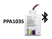
It is a power pack that provides 12V DC output to power sensors and switching for non-dim-to-off LED drivers. The PPA103S also provides a 0-10V dimming wire for bi-level motion control and relay output.
