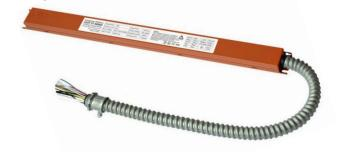
The BLD-YTXXD-XXX series LED Emergency Driver is UL listed for field and factory installations. It switches to emergency mode during power failures, providing up to 90 minutes of lighting. With an integrated battery, charger, and converter, it delivers 8 or 15W constant power at 30-60VDC. Its slim shape is ideal for use in linear LED lighting fixtures.
