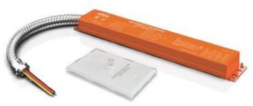
The BLD-HMXXD-YYY series LED Emergency Driver is UL listed for field and factory installations. It switches to emergency mode during power failures, providing up to 90 minutes of lighting. With an integrated battery, charger, and converter, it delivers 6-25W constant power at 170VDC. Ideal for 0-10V dimmable indoor commercial LED fixtures, such as flat panels, troffers, downlights, and linear strip lights.
