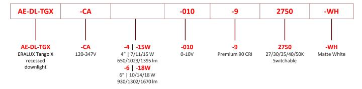
Fixture Family Input Voltage Size | Power Dimming CRI CCT Finish
