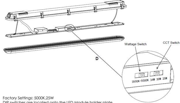
DIP switches are located onto the LED Module holder plate temperatures and 3 powers respectively, which can perform the desired color temperature and lumen output combination.
