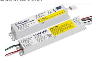
This LED Emergency Driver from Streamer is UL listed, and it is factory installed. It switches to emergency mode during power failures, providing up to 90 minutes of lighting. With an integrated battery, charger, and converter, it delivers 8W constant power at 50-180VDC. Its slim shape is ideal for use in linear strip lighting fixtures.
